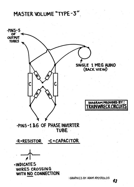
**The Trainwreck Master Volume Type-3** adds a 1MA pot that simply mixes the two mirror image audio streams from the phase inverter together. The two streams will cancel each other out. This master volume is very easy to try by simply alligator clipping in a 1MA pot. I installed this master volume in my 5F6A clone and I'm very happy with its performance. Rob Robinette
