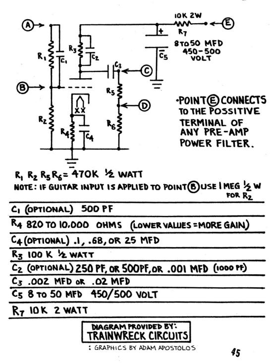
**The Trainwreck Universal Gain Stage** is a very flexible circuit due to its voltage dividers at the circuit's input and output.
