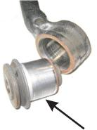
Factory bushing metal shell must be pressed out of upper control arm for Energy Suspension polyurethane bushings to fit properly.
