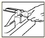
Step 3. Lubricate nipple and socket threads. Use a molydisulfide base lubricant for stainless steel fittings (e.g. Molykote Type G); lubricants containing chloride are not recommended. Other material combinations use standard petroleum lubricants. Hold the nipple with hex in the vise. Push hose over nipple with twisting motion until seated against nipple chamfer. Push socket forward and start threading of socket to nipple.
