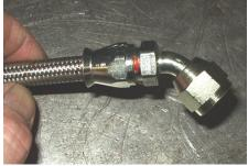
this point. You may now back the hose end out of the hose up to one full turn to orient it in the direction desired. Doesn't this have to be tight? NO! The initial torque down crushes the brass ferrule down a few thousandths, which seals the teflon liner very well against the male nipple of the hose end, which means that you will still seal the joint positively even if unscrewed up to three full turns (!). These lines seal so well that they can also be used with Nitrous without fear of leakage!
