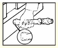
Step 2. Push the sleeve over the end of the tube and under the wire braid by hand.
