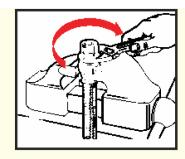
Step 4. Wrench tighten hex until clearance with socket hex is at .031 inches. Your thumbnail is a convenient measuring device. Tighten further to align corners of nipple and socket hexes. CLEAN, PROOFTEST TOTWICE OPERATING PRESSURE AND INSPECT ALL ASSEMBLIES.
